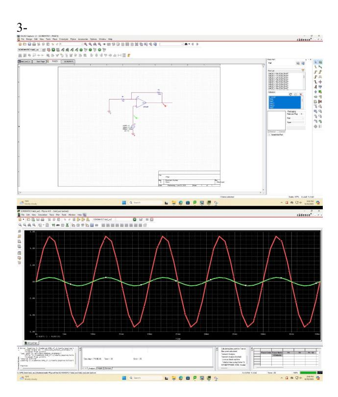
According to the manual calculation, the gain of non inverting amplifier should be 11, and it can be seen in the oscilloscope and simulation that the output waveform is 11 times amplified. Then as the name suggests, output will be non inverted as compared to input which means it will in phase with the input which is also evident in the graphs.
