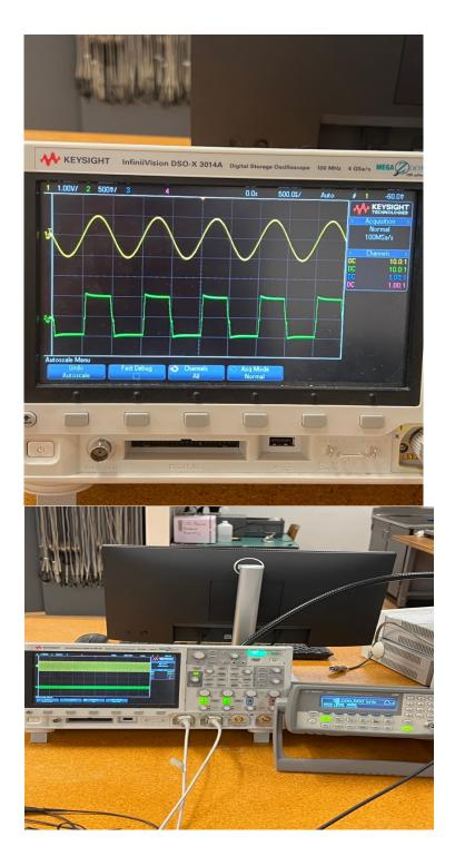
We calculated the values of resistors and capacitors based on the cutoff frequency of 2khz. For a low pass filter, whenever the signal of less than 2khz is passed, it will allow it. But when signal is out of the band, it will attenuate it.
